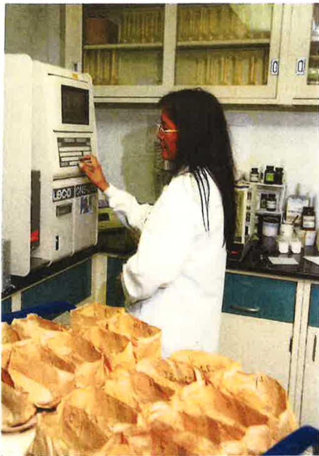
Analyzing alfalfa: Marjorie Yazzie uses a carbon, nitrogen and sulfur forage analyzer to test alfalfa quality at the Navajo Agricultural Products Industry's Agricultural Testing and Research Lab.
